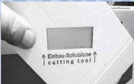
Please don't just throw away the inner packaging, as it is designed to be used as a template for marking the switch aperture on the model. Cut the opening using a knife or saw, working slightly outside the marked line (see photo).
