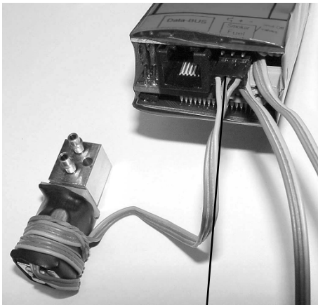
Fuelvalve to be connected on lower output
